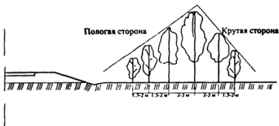
Fig. 1. Scheme of noise-gas and dustproof plants
