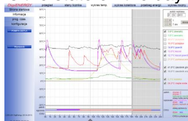
Figure 2. A screenshot of the temperatures of the flows of the heat carrier and water in the plant at real time.
